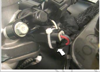
**NOTE:** Acting as a strain relief, cable strap allows connector conduit to be flexed without putting stress on terminal connections. Movement or vibration of conduit without cable strap may cause eventual component failure.
