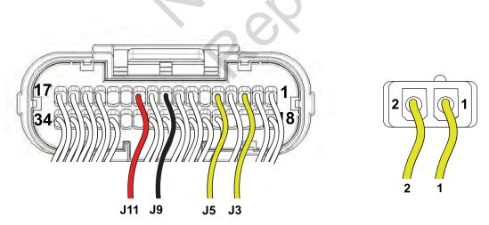
Stator Power Connector (Stator Side)
