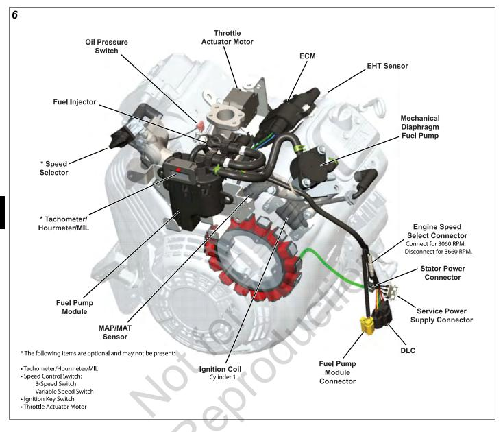
NOTE: Air cleaner assembly and fuel pump module cover removed for illustration purposes.
