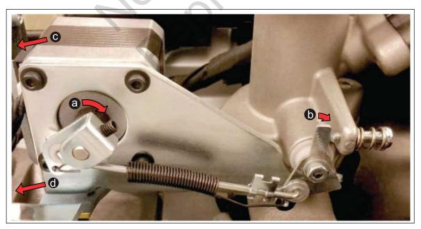
Verify Proper Installation of Throttle Actuator Motor Lever and Linkage.
