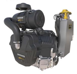
The engine is equipped with the Oil Guard System that features a five-quart reservoir for oil storage and extends the oil change interval to 500 hours. The system works by moving oil continuously between the engine and the reservoir, storing oil away from engine heat. This feature, along with a 192 oz. system capacity, minimizes thermal breakdown to extend the life of the oil and protect the engine better.
