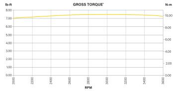
All power (HP) and torque (Nm) levels are stated Gross per SAE J1940 as rated by Briggs & Stratton
