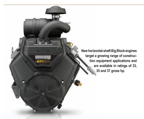
ice life; automotive-type JCC AC8A alloy pistons with a three-ring ring pack and a chrome-plated top compression ring designed for high durability and improved oil control; dynamically balanced ductile-iron crankshafts and connecting rods with larger bearing surfaces, both of which are designed to yield durability and longevity; 5.0 in. Donaldson cyclonic air cleaners intended to improve intake-air-filtration efficiency; and full-pressure lubrication systems with spin-on oil filters.
