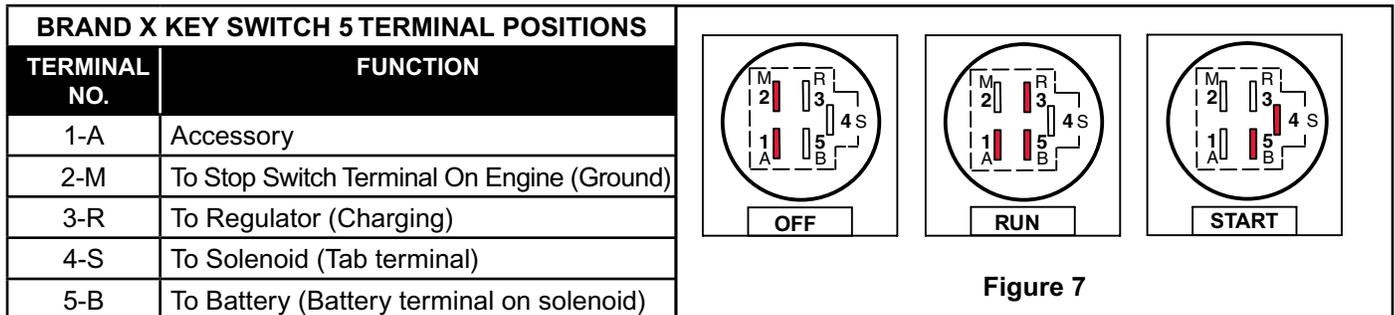
It is not possible to show all of the wiring diagrams or keyswitch combinations that are used by equipment manufacturers. However, the following wiring diagrams for the most popular Briggs & Stratton engines may be used as a guide when replacing an engine. The wiring diagrams show the type of keyswitch that is compatible with the alternator system shown.
