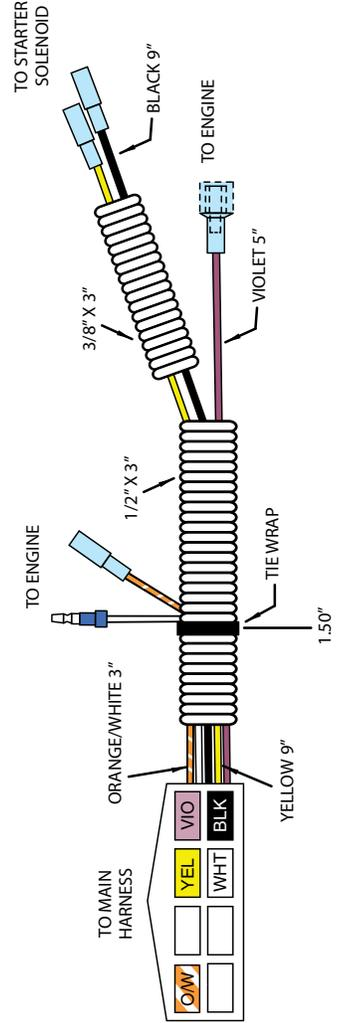
**ALTERNATOR HARNESS AND REPAIR LEADS**
