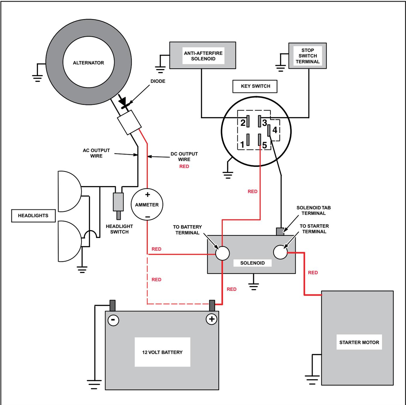
Typical Dual Circuit Alternator
