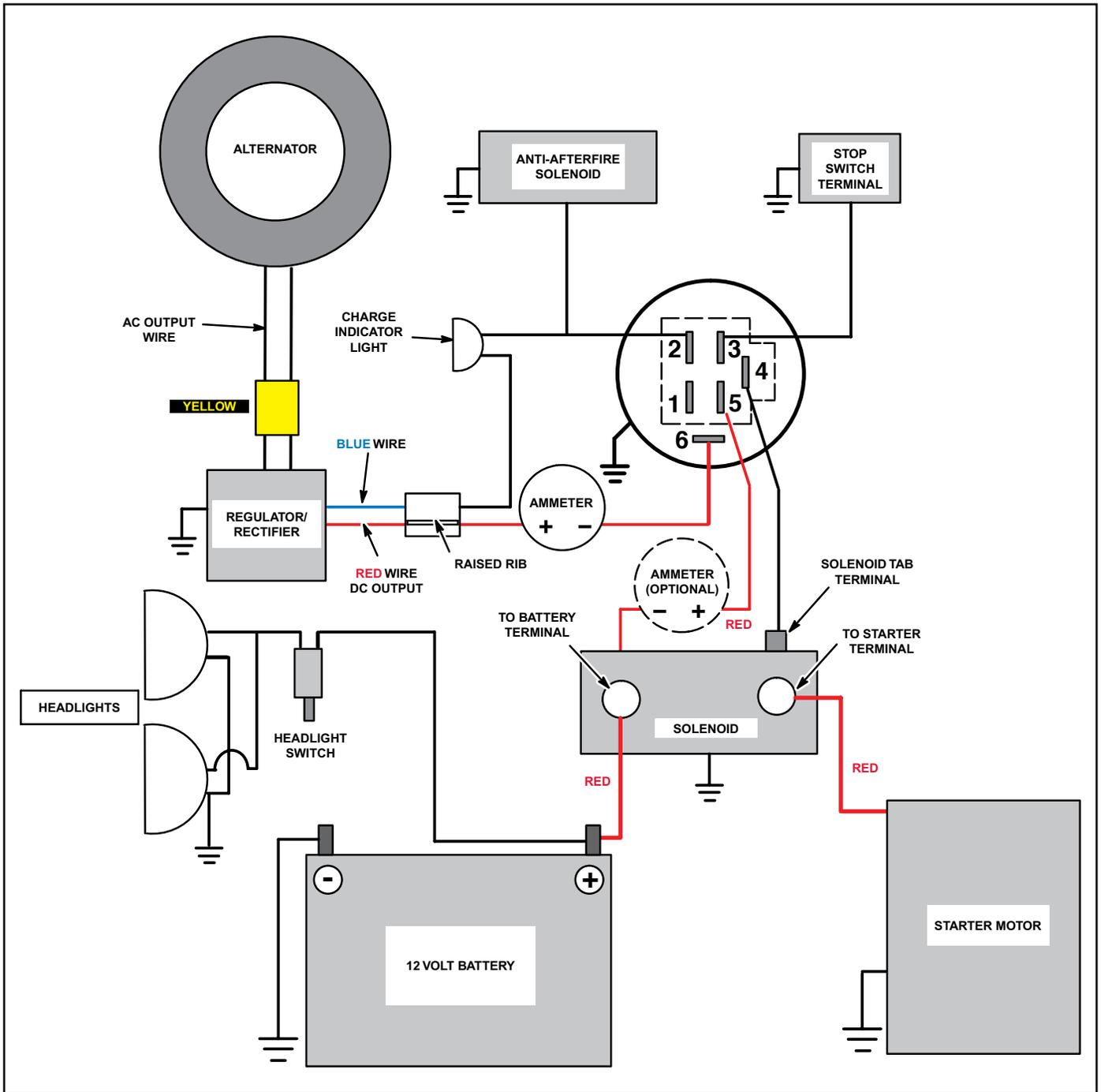
**Typical 16 Amp Regulated Alternator Wiring Diagram
