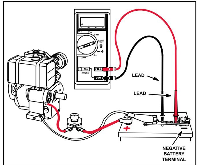
2. Insert RED test lead into  $v \Omega \rightarrow$  receptacle in meter and RED receptacle on shunt.
