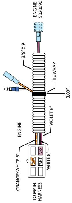
**FERRIS®/SNAPPER® PRO ENGINE TO EQUIPMENT WIRE HARNESS**
