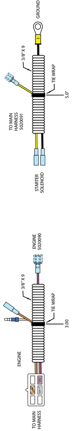
**FERRIS®/SNAPPER PRO® ENGINE TO EQUIPMENT WIRE HARNESS**
