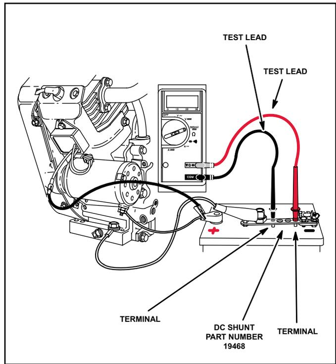
**DC Amperage Output Check
