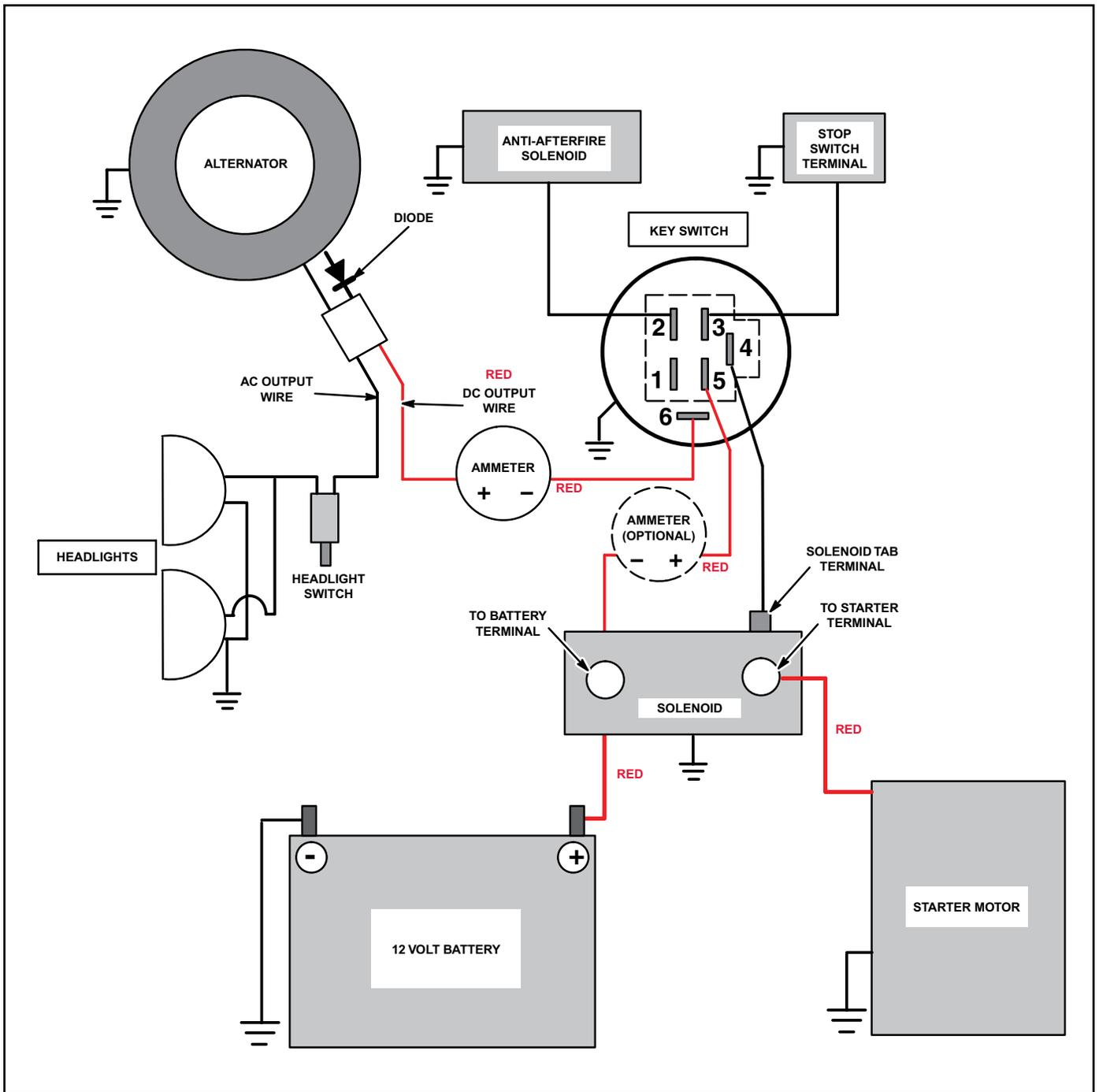
**Typical Dual Circuit Alternator
