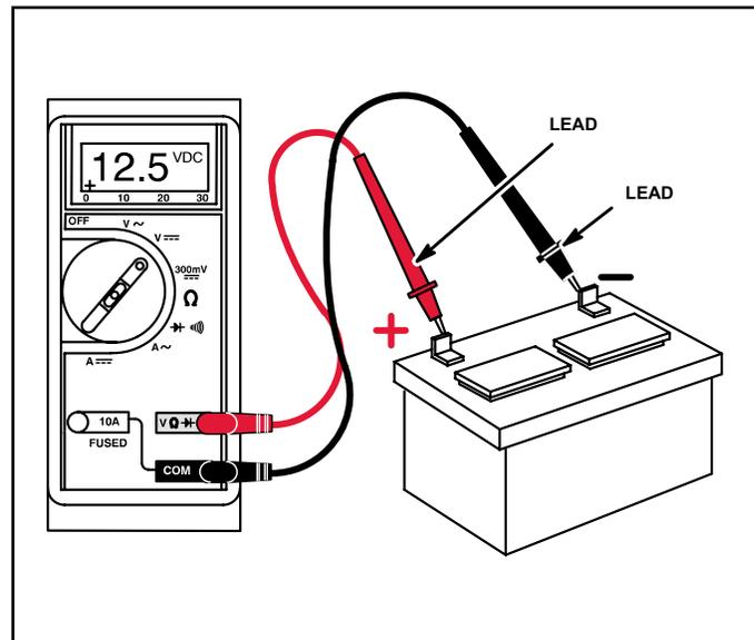
DC Voltage Battery Test
