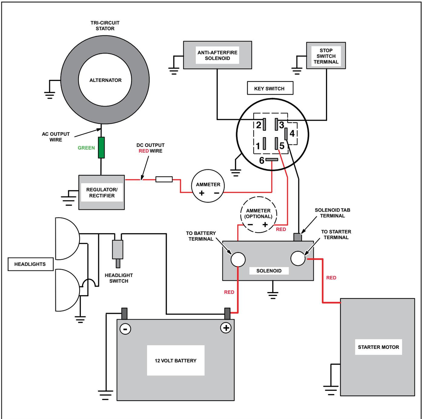
**Typical 5/9 Amp Regulated Alternator Wiring Diagram
